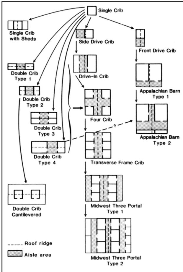
These drawings demonstrate a conjectured evolution of crib barn floor plans. The transverse frame crib is one of the most common types in Georgia. (Illustration courtesy of M. Margaret Geib and the University of Massachusetts Press, from Nobel and Cleek 1995).
