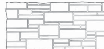
RANDOM BROKEN COURSED ASHLAR
