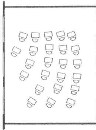
B - CURVED ROWS TO MAINTAIN FOR EACH PUPIL A 50-DEGREE ANGLE BETWEEN LINE OF VISION AND FRONT LIMIT OF WINDOWS
