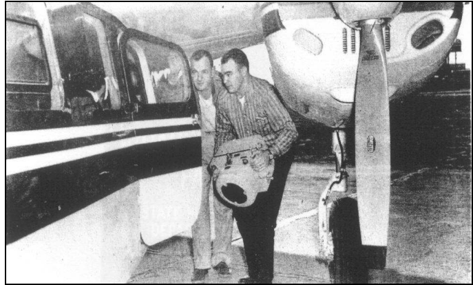
Figure 6. Georgia State Highway Department employees load a camera on the department's airplane. Aerial photography eliminated the need for labor intensive ground surveys and was one of the new technologies employed to improve the efficiency of locating and designing interstate highways. Source: Georgia Highways (Jan. 1958).
