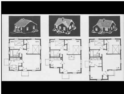
And this diagram — a little easier to see — shows how the basic American Small House plan-form could be adjusted to create two additional and slightly larger versions which appear to be quite common here in Georgia:
