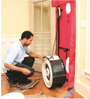
Man conducting blower door test as required by Georgia energy code.
