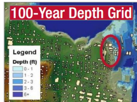
Figure 1. Example of Use of Depth Grids in Floodplain Mapping (not Glynn County)
