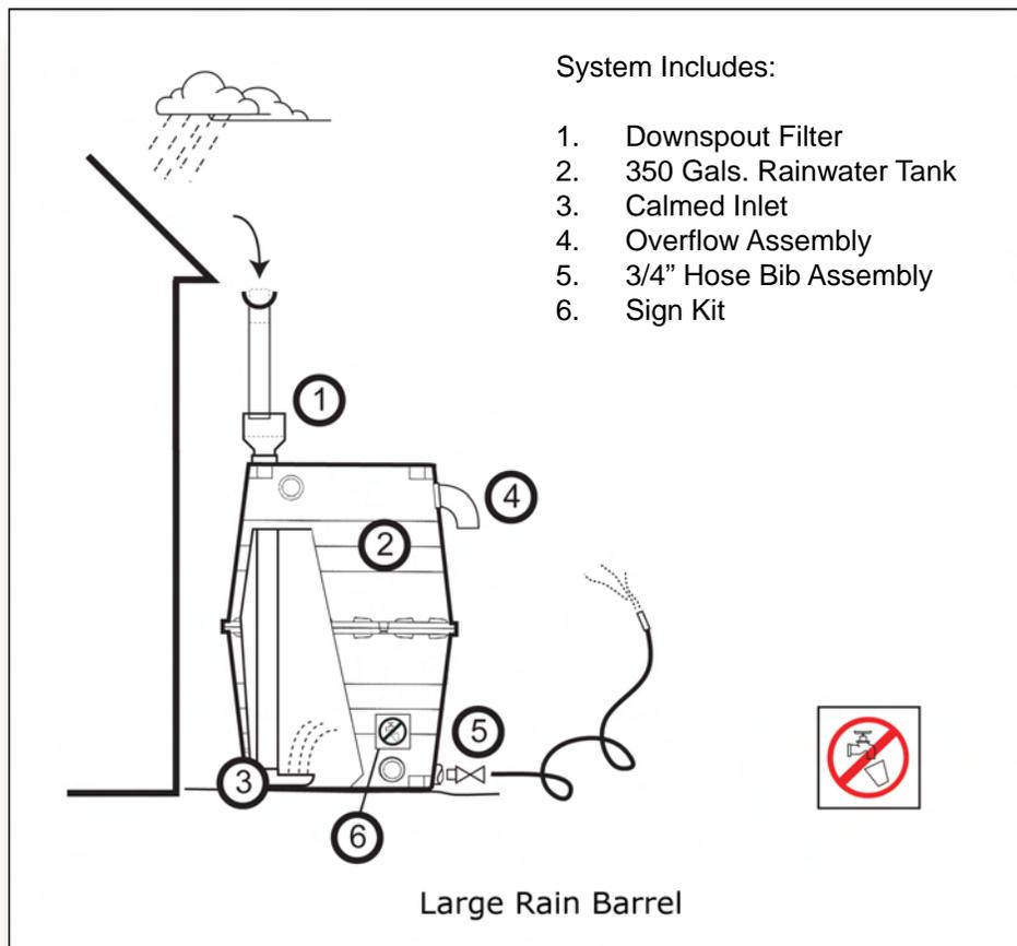
Figure 4.9 Schematic for 350 gallon rain barrel
