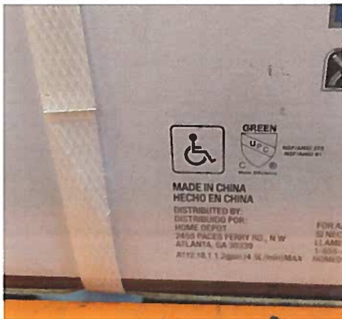
Bottom of lavatory faucet box showing 1.2 gpm flow rate
