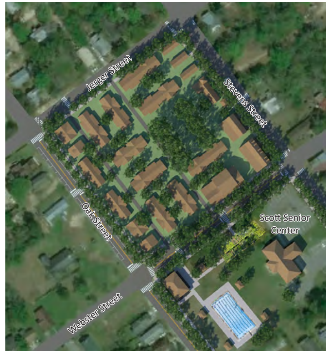
Strategic Upgrades Site Plan: The existing vehicle circulation is maintained along with the common space. New buildings replace the existing structures at the corners.
