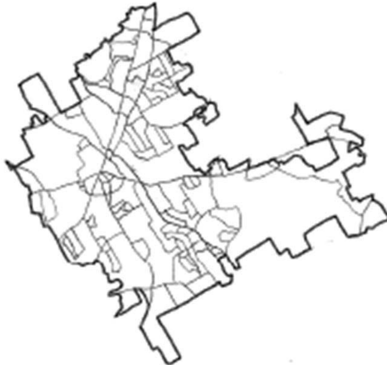
Figure 8-5: Street Connectivity – Roads in Snellville that have more than one Access Point
