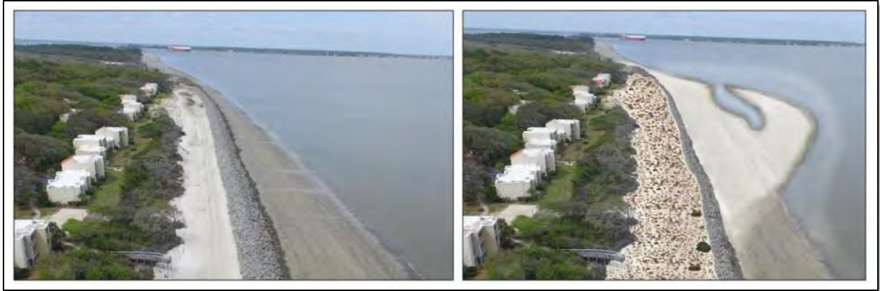
Figure 5.13: "Sand Motor" Project Visualization – Nearshore Placement
