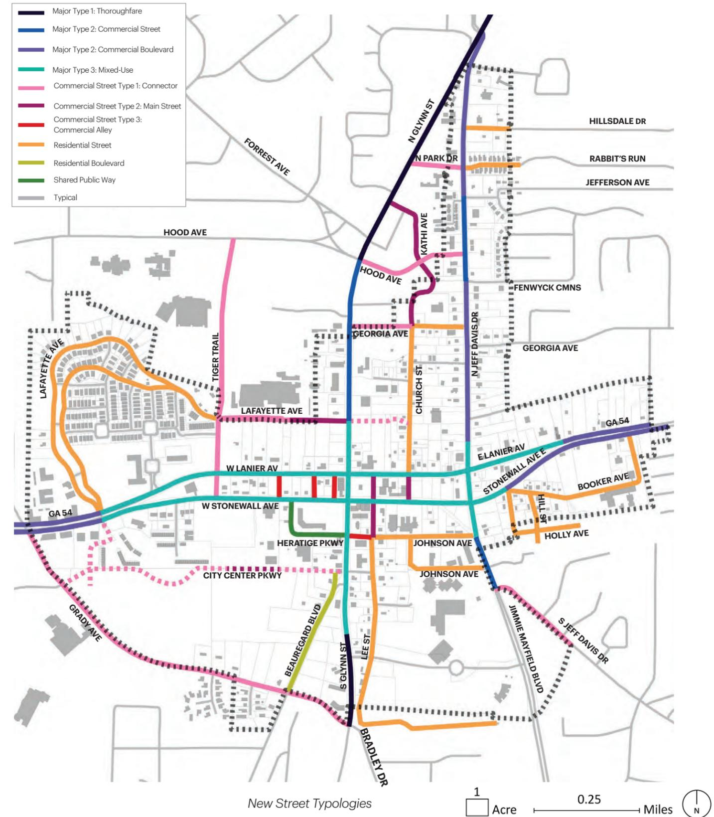
The UDO street hierarchy establishes prerequisite minimums for roadway and street design to include dimensional requirements for right-of-way (ROW), surface pavement, and sidewalks. The UDO street hierarchy also establishes access requirements. It is within the boundaries of the UDO street hierarchy and typologies that the Fayetteville LCI's proposed Mobility Framework sits.
