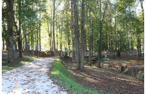
Root bridging insures protection of existing trees and allows the trail to blend into a wooded setting.
