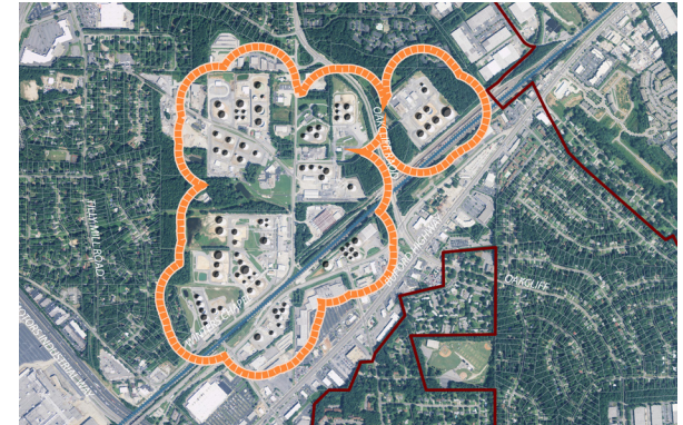
Proposed safety area around tank farm structures
