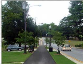
Example of multi-use trail. Site furnishings along trail include decorative benches, trash receptacles and pedestrian-scale lighting. Planted landscape strip provides separation between vehicular and pedestrian traffic.
