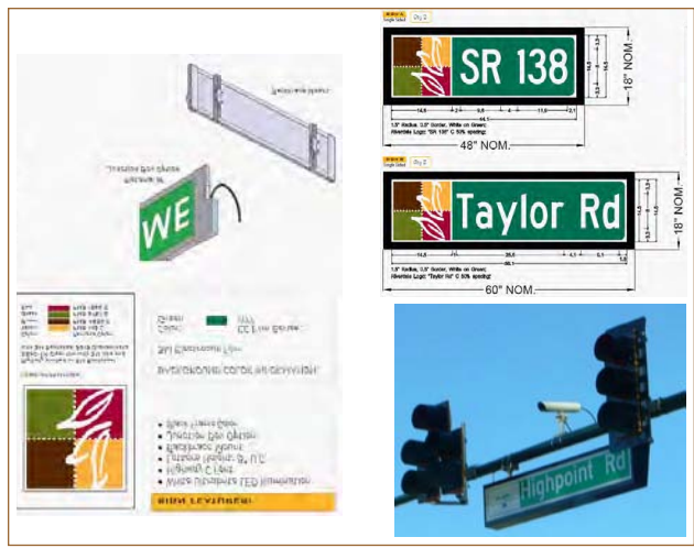
Street name signs with internal lighting
