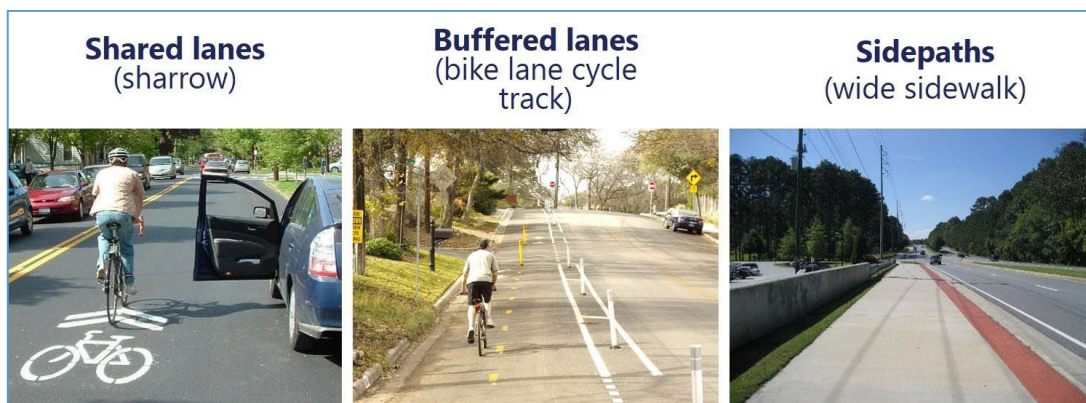
FIGURE 26. BIKEWAY FACILITY EXAMPLES
