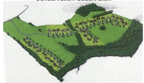
Same number of homes, less linear feet of roads and utilities; more open space
