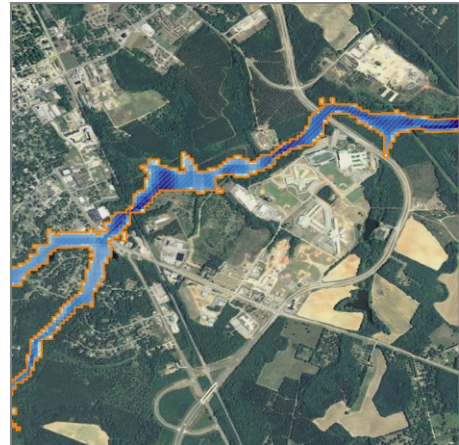
Figure 4. DCA can generate flood depth grids to illustrate the potential extent of flooding in a community
