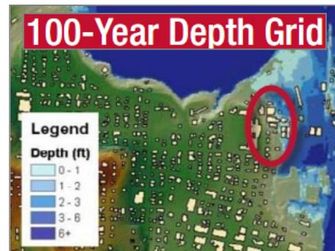
Figure 1. Example of Use of Depth Grids in Floodplain Mapping (not Carroll County)
