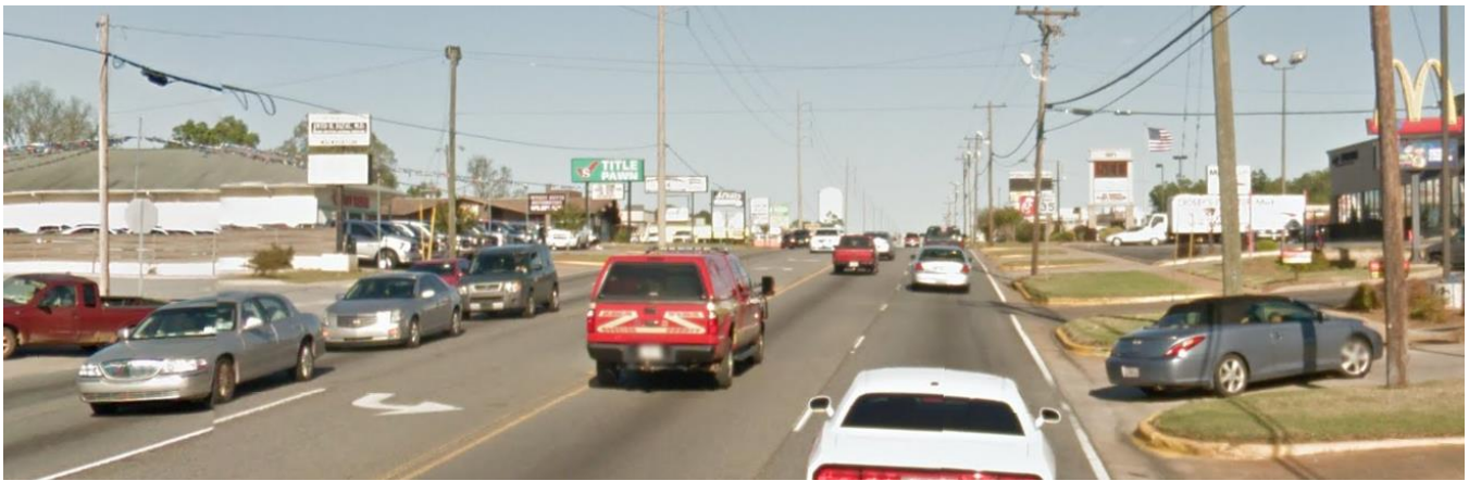
Figure 23 – Watson Boulevard in Warner Robins, pictured here near Houston Road, is a prime example of in-town corridors where commercial strip development has become the dominant land use. Note the 35mph speed limit posted on this major thoroughfare, which is necessitated by the multiple points of ingress and egress for traffic at each establishment. In this photo, there are six curb cuts within approximately 400 feet of distance on the right side of the road. There is also no bike lane and limited amenities which can be reached on foot. As such, travel by automobile is the only practical option along this route.
