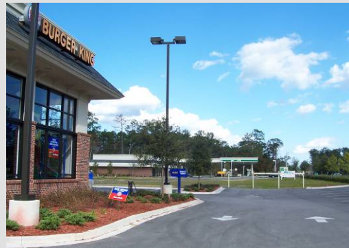
Cross-access easements allow existing and future development to share on-site travel lanes while reducing the need for multiple curb cuts on the highway.
