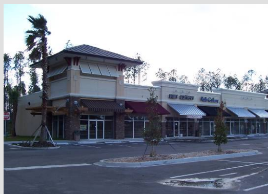
Landscaped islands can be incorporated into site design to manage on-site traffic and reduce impervious surfaces.
