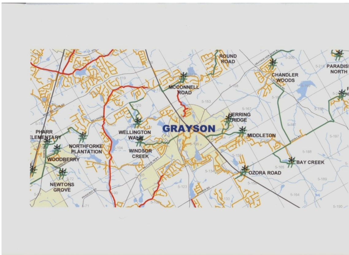
Grayson Area Existing Sanitary Sewer, August 2008
