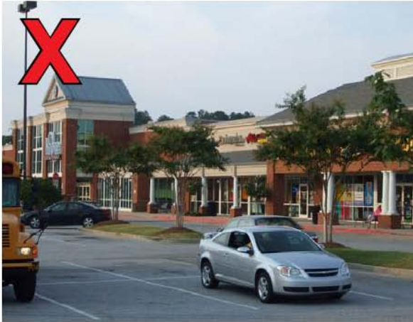
(Top Left) Avoid landscape that is out of scale with development and corridor. This results in blocked signage of commercial buildings and little shade for large surface parking lots.
