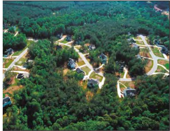
An example of a conservation subdivision, which maximizes and protects existing green space/trees via site design
