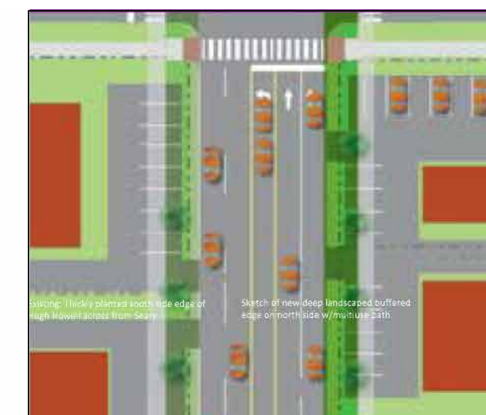
Relocated Parking Frees Space for ROW Acquisition
