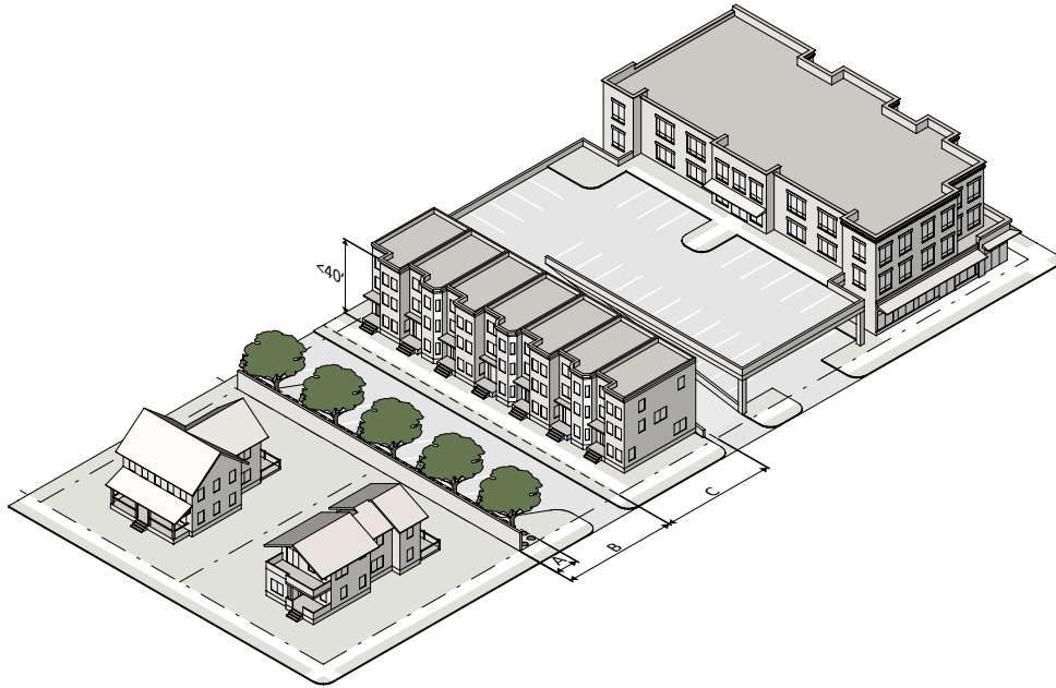
Diagram illustrating land use transitions, from multifamily to townhomes to single family homes.
