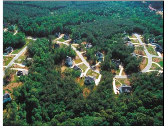
An example of a conservation subdivision, also known as an open space subdivision, which maximizes and protects existing green space/trees and reduces impervious cover, soil erosion and infrastructure costs
