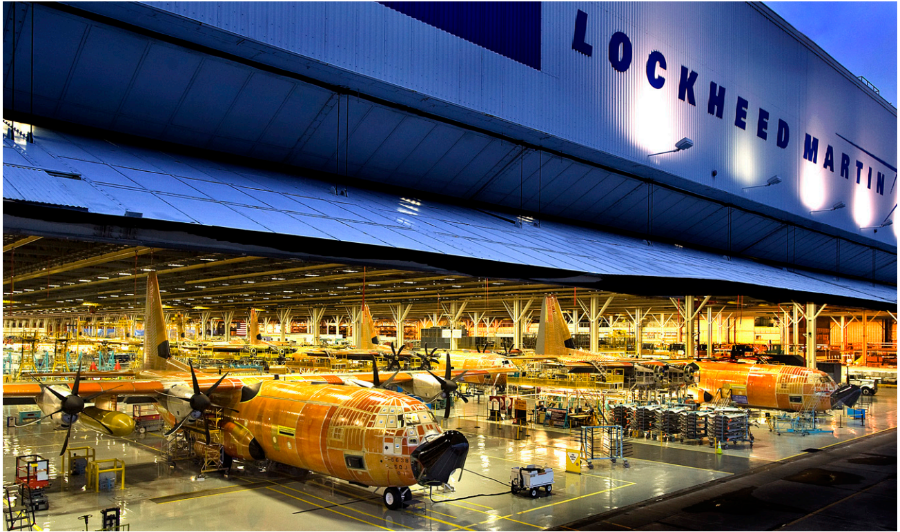
The C-130 Production line in Marietta (Image courtesy of Lockheed Martin Corporation)
