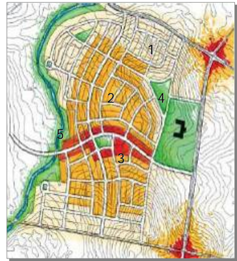
TND form: (1) Lower-density residential, (2) urban residential, (3) Mixed-Use center, (4) Open Space and Civic Site, (5) Linear Park.
