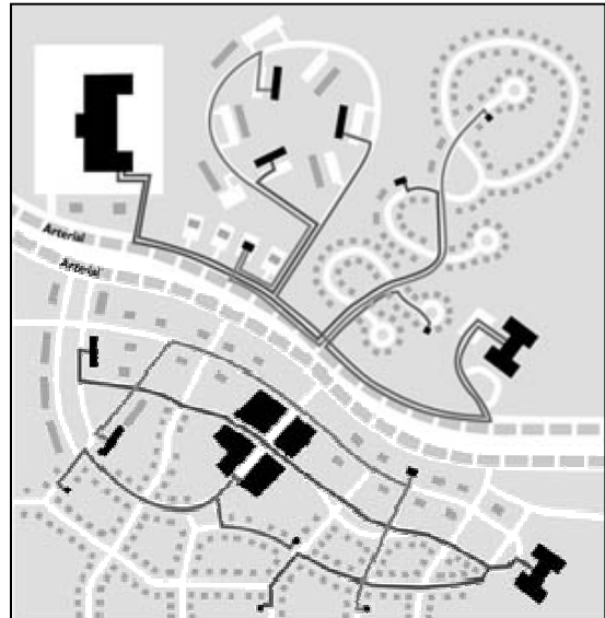
Developing Suburban character area seeks to encourage the development pattern described on the bottom of the diagram and discourages conventional suburban sprawl shown in the top of the diagram.
