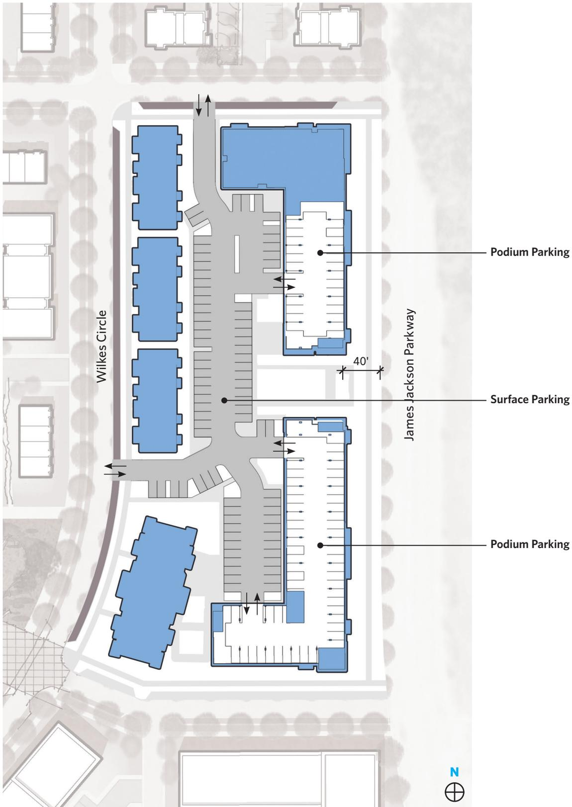
**Phase I Parking & Circulation Plan** A portion of the parking spaces will be provided in ground floor podium under the two corridor buildings. The remainder of the parking spaces will be provided in a surface lot in the center of the development block.
