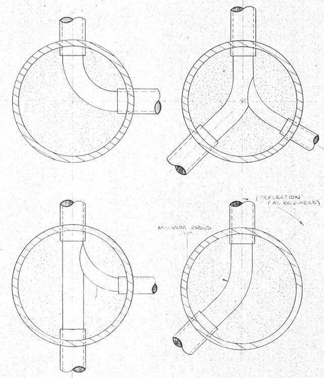
NOTE: INVERTS CONSTRUCTED AT 1/8" DROP ACROSS THE SIDE OF MANHOLE
