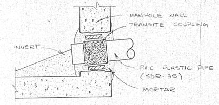
NOTE: ALL PVC PLASTIC GRAVITY SEWER MAINS ENTERING MANHOLE WALL SHALL BE GROUTED IN PLACE WITH A TRANSITE COUPLING
