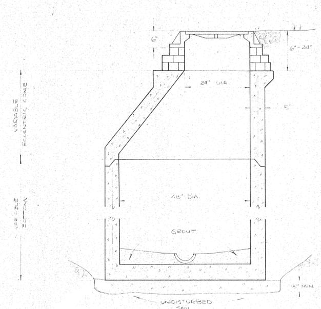
**MANHOLE STANDARD CONSTRUCTION (CLOSED BOTTOM)**
