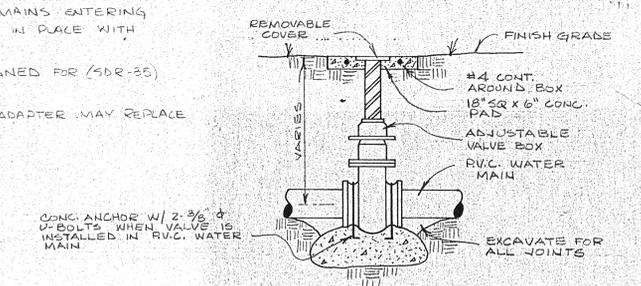
**TYPICAL GATE VALVE INSTALLATION**
