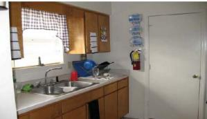
Each unit has a living room/living area, kitchen, bedroom(s), and bathroom(s). The floors in the units are a combination of carpet and vinyl tile. Windows are vinyl framed casement units. Exterior doors are metal; interior doors are hollow core wood. Interior walls are painted drywall; ceilings are painted drywall. Ceiling height is generally 8 feet. Hot water is supplied via individual water heaters.
