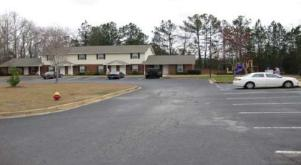
The buildings have a poured concrete foundation. The buildings have a combination brick and siding exterior, and a pitched roof covered with shingles.
