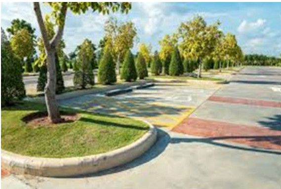
Planting landscaped tree islands in paved parking areas provides shade and mitigates heat island effects. The use of pervious surfaces reduces stormwater runoff and keeps community drainage systems from being overloaded.
