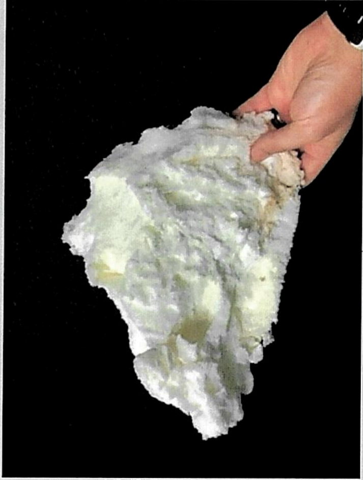
Outside facing of spray foam
