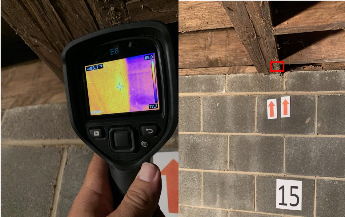
Photograph 2. Image of the IR camera screen (Flir E6) indicating an area determined to show termite activity during the first inspection (July, 17) and a visual image of the same area indicated by the red box (right).
