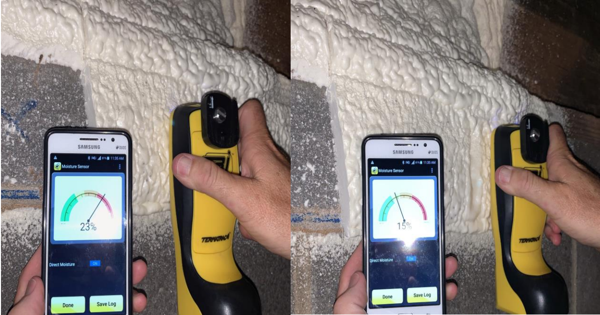
Photograph 6. Image of the Termatrac T3i percent moisture readings on closed-cell foam at Location 5 on the block in an area with (left) and without (right) termite activity.
