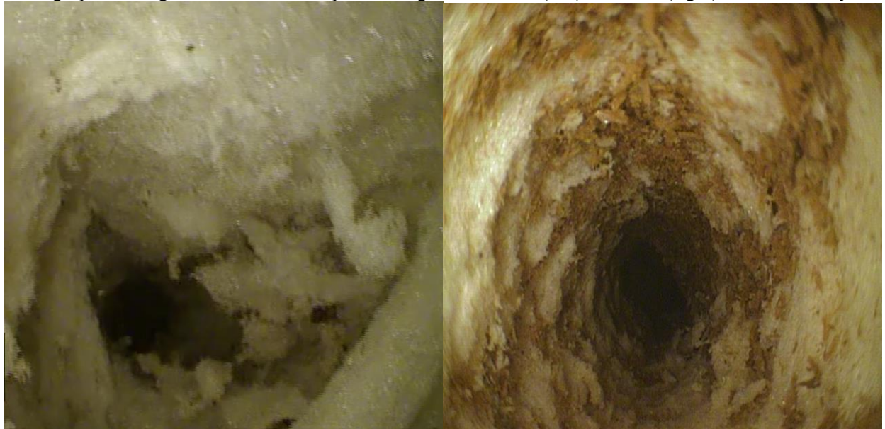
Photograph 5. Images from the borescope showing SPF without (left) and with (right) termite activity.
