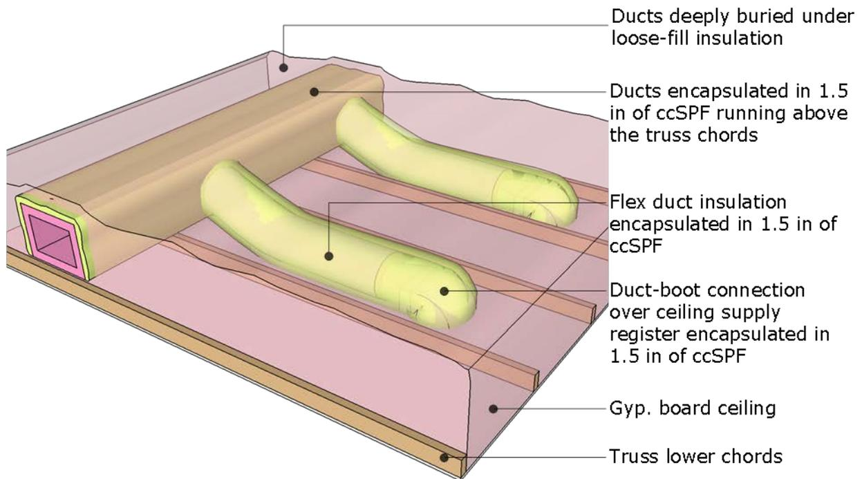
**Figure 4. Detail of buried and encapsulated duct**
