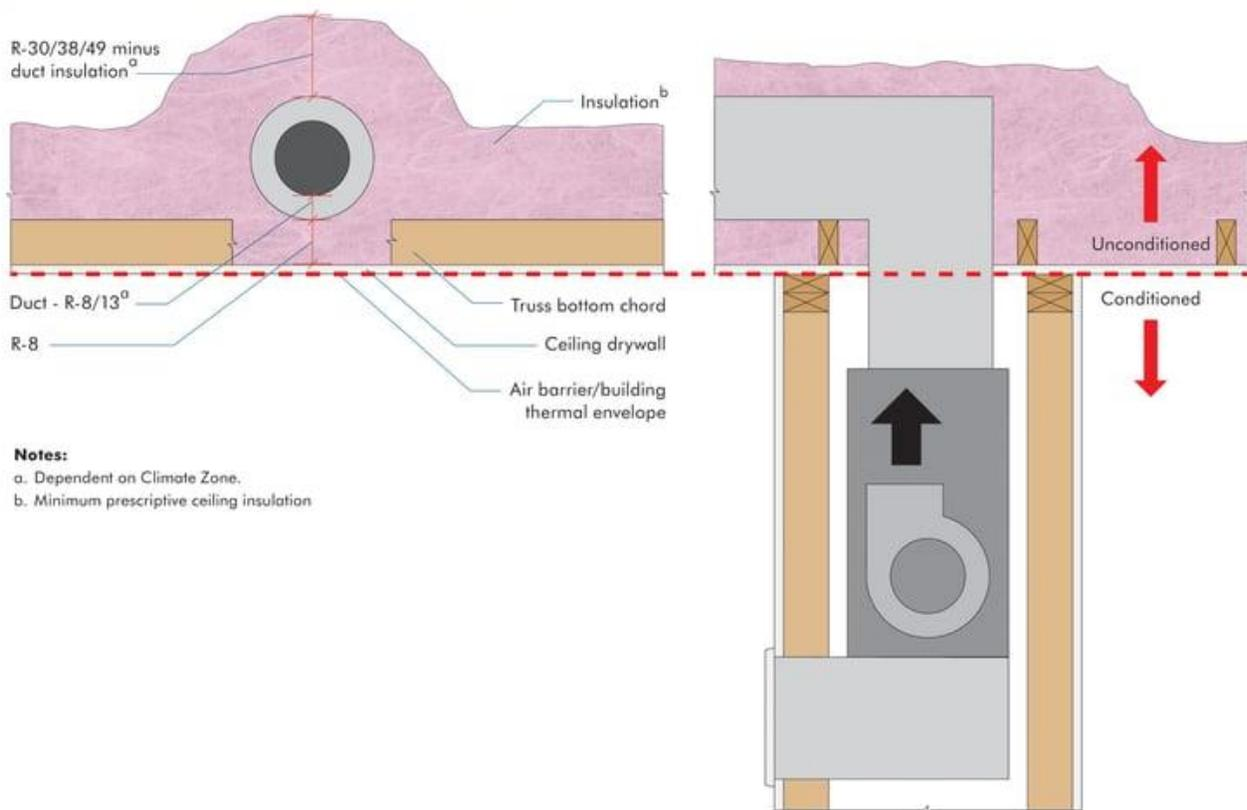
When incorporating these buried duct options they must be installed carefully so as to avoid condensation problems. While all applicable IRC duct requirements must be followed, making sure the vapor retarder on the duct insulation remains sealed, duct leakage limits are not exceeded, and that consistent minimum insulation levels around ducts are maintained will help minimize the potential for condensation with buried ducts.
