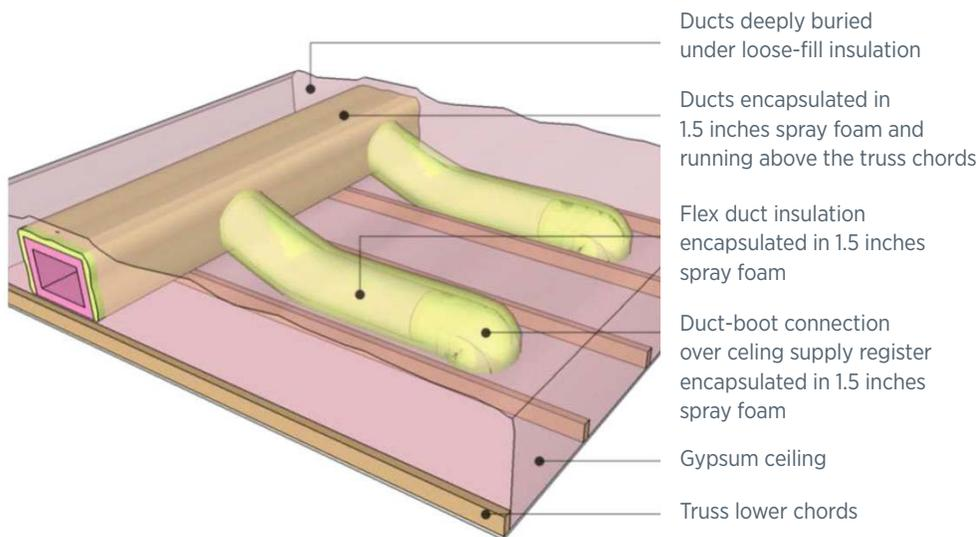
BEDs are first encapsulated with closed-cell spray foam insulation, then buried under loose-fill insulation. Initially conceived as a way to apply the buried-ducts concept to humid climates (where condensation could occur on the outer surface of buried ducts). Encapsulating the ducts in spray foam is a high-performance duct insulation strategy that can be used in all climates.
