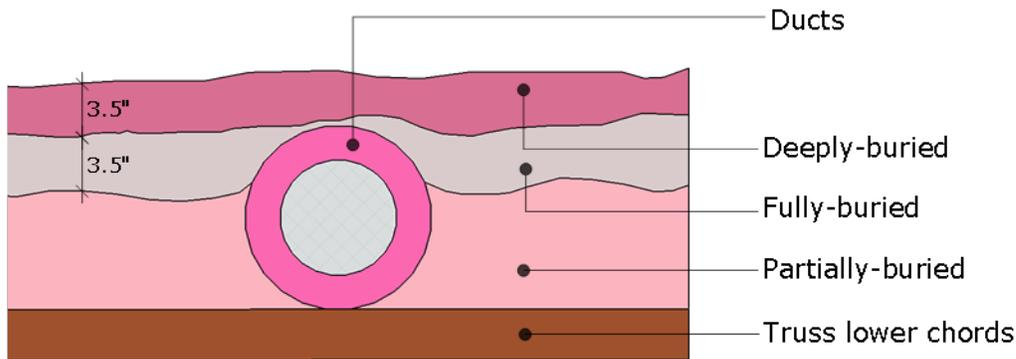
**Figure 42. Diagram of buried duct modeling configuration**
