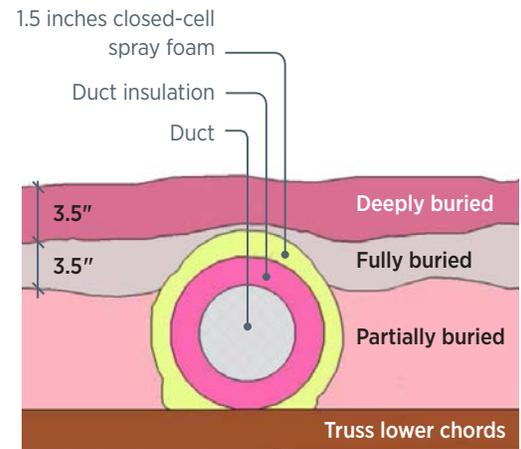
Building America research shows encapsulating the ducts in spray foam before covering with loose-fill insulation provides adequate protection against condensation making this low-cost, high-performance method appropriate for every climate zone.
