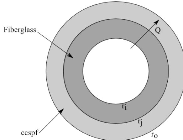
**Figure 41. Flexible ductwork encapsulated in ccSPF**
