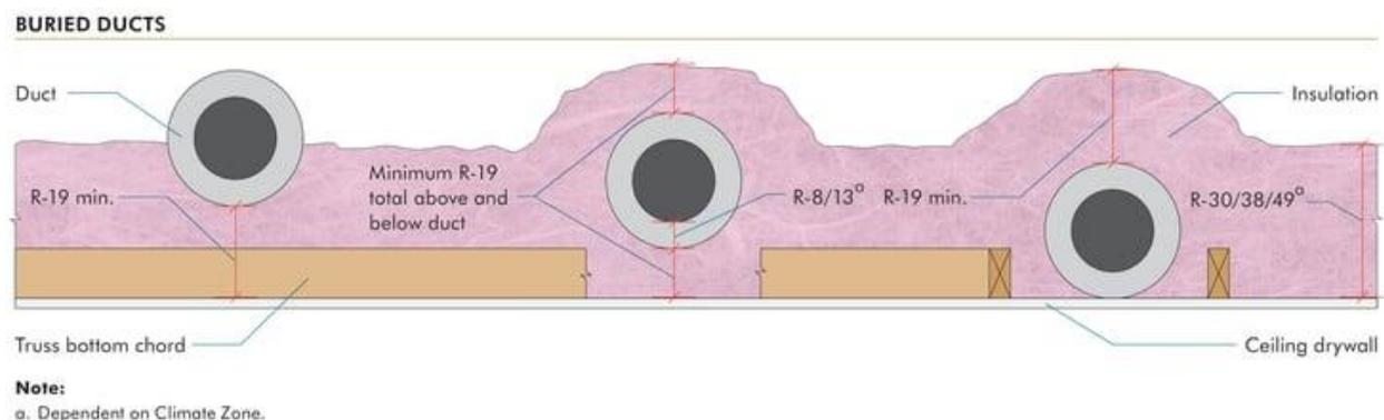
The 2018 IECC/IRC also permits buried ducts to be modeled as being insulated to an effective R-25 level or be modeled as being within the conditioned space of the building.
