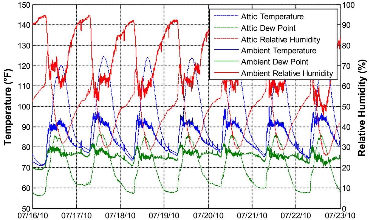
**Figure 52. Pre-retrofit ambient and attic conditions at House 1**
