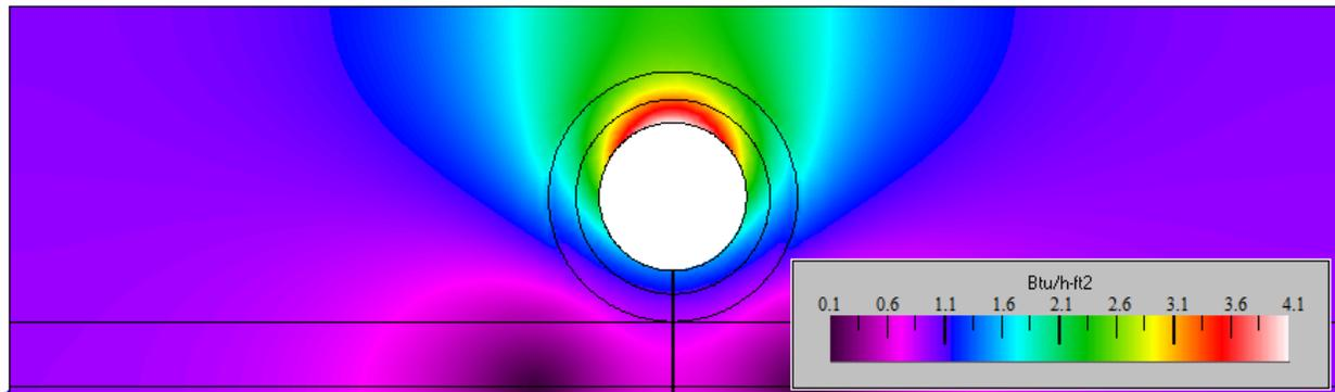
Figure 44. Heat flux magnitude through encapsulated and fully buried 8-in. diameter duct
