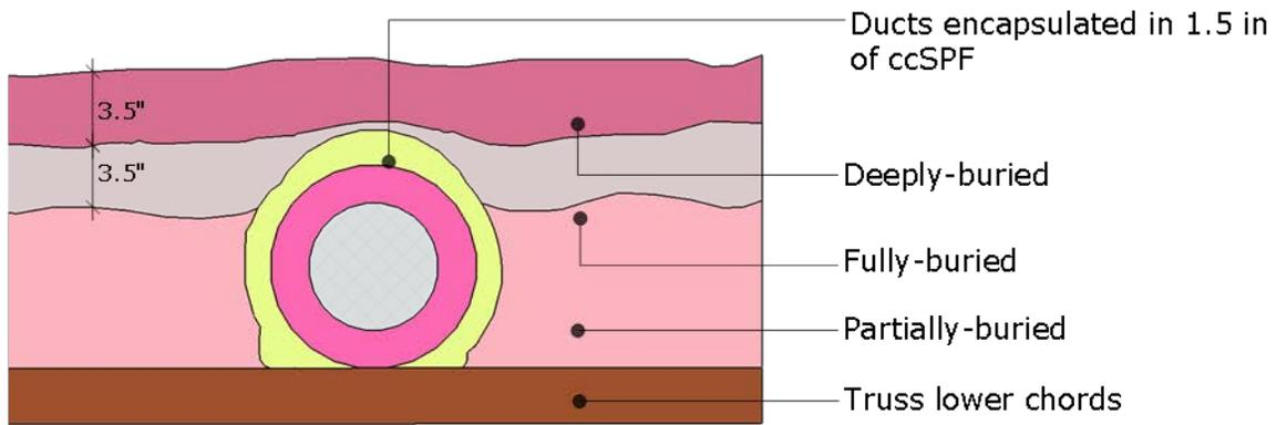
Figure 43. Diagram of buried and encapsulated ducts
